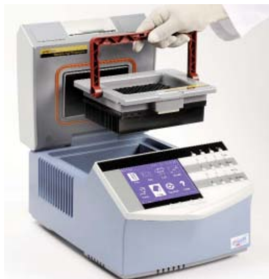
Thermal cycler door open with a heater system on the back side of the door to avoid condensations.
