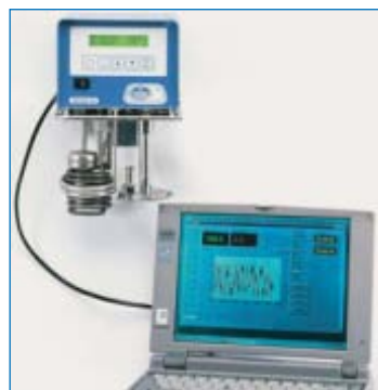
Units with a RS-232 connection can be controlled by a computer and can print out parameters.
