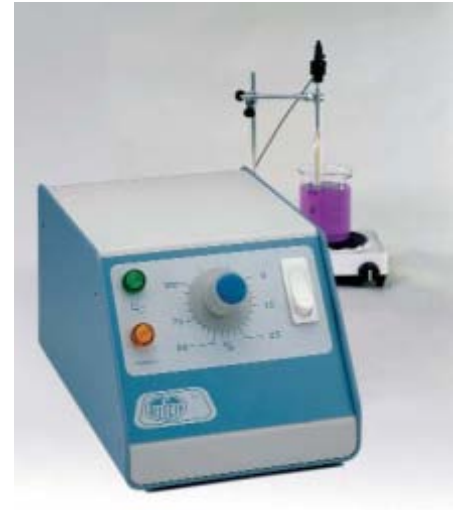
“Enertron” application to a hotplate, showing the unit connected with an electronic contact thermometer.
