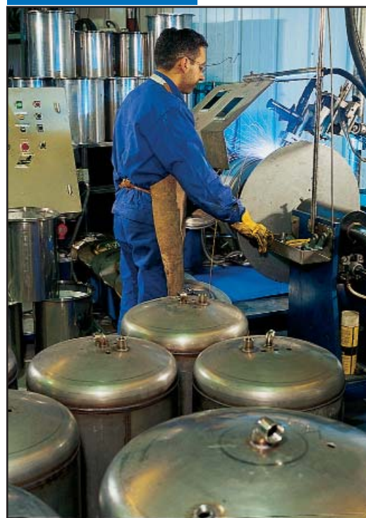
Circular welding for pressure and vacuum vessels.
