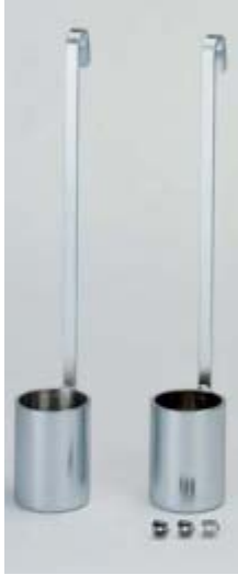
Flow cups with handle. Models DIN 53211 N° 4 and Ford ASTM D-1200.
