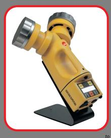
DUO SAS-SUPER 360 is a single body air sampler with two aspirating heads: two different media types can be used for simultaneous samples. 1000 litres of air can be sampled in less than 3 minutes. These are the revolutionary specifications of the new DUO SAS SUPER 360 microbiological air sampler produced by International Pbi.
