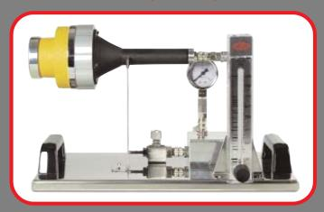
"Pinocchio Super" is used to test the microbiological quality of compressed air and gas used in Clean Rooms according to ISO 8573/7.
