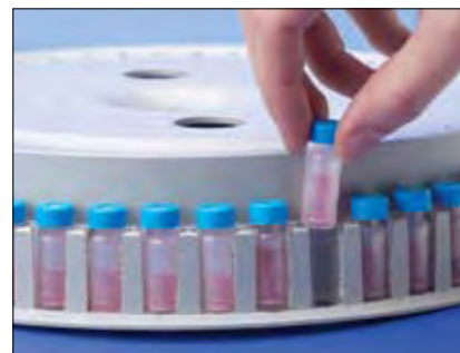
Mini-UniPrep in an HPLC autosampler
