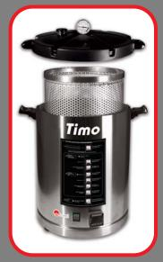
"TIMO" produced by International PBI, according to the "PED" European Standard, is a 23 litres portable autoclave suitable for the microbiological laboratories that have space problems. The structure is made in AISI 304 stainless steel and the requested space is only thirty frontal centimetres. It can be positioned on floor or laboratory bench. It does not need a water connection. The vertical construction guarantees the complete use of the sterilisation chamber.
