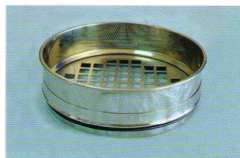
Tamiz inoxidable con chapa perforada de agujero cuadrado St. steel sieve with square perforated plate
